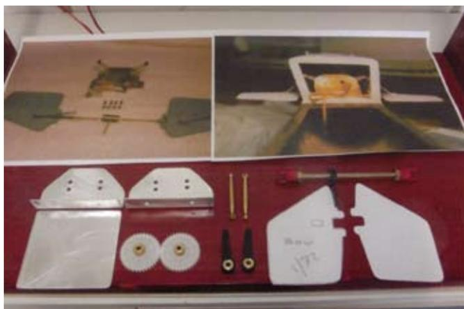
**Components for the bow planes and mechanism**
