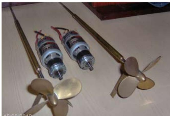
*The main drive motors, props and prop shafts*
