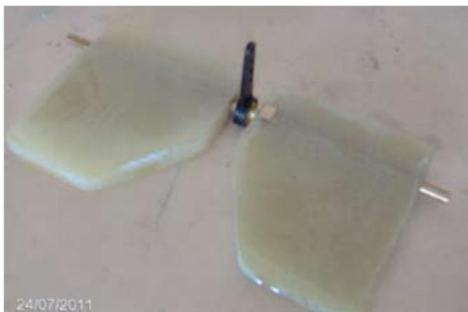
**Completed stern planes with control mechanism**
