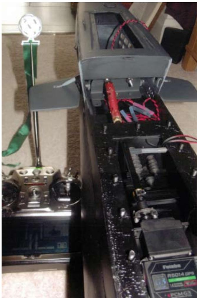
*The servo and shaft for operating the bow planes*
