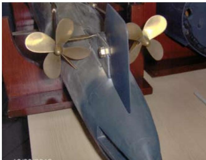
*A view of the stern with the props and shafts in place*
