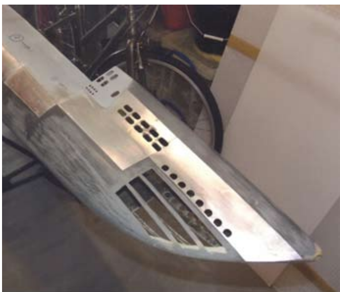
The internal bulkheads with the carbon and brass joiners
